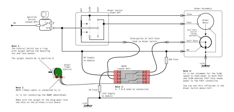
1/ Connect terminal 1 to +12V power, after the ignition switch, using the supplied 2A fuse and fuse holder.
