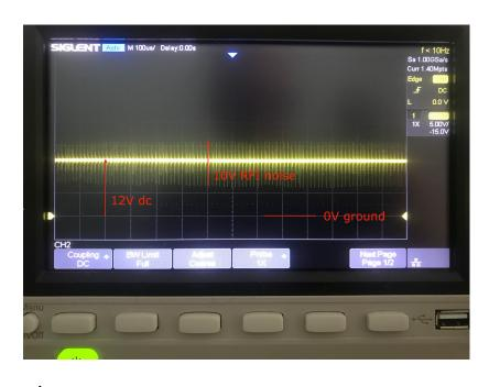
If the source of the interference can not be readily identified & remedied, it may be necessary to install an inline Suppressor to the red/black lead which supplies +12V to the Module's circuit board.
