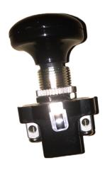
In order to fit the switch to your dashboard or bracket the mushroom button must be removed: Hold the switch body & gently twist the mushroom button 1/4 turn anticlockwise. Refitting the mushroom button is the reverse of this operation. (The same method is used if the LED needs replacing).
