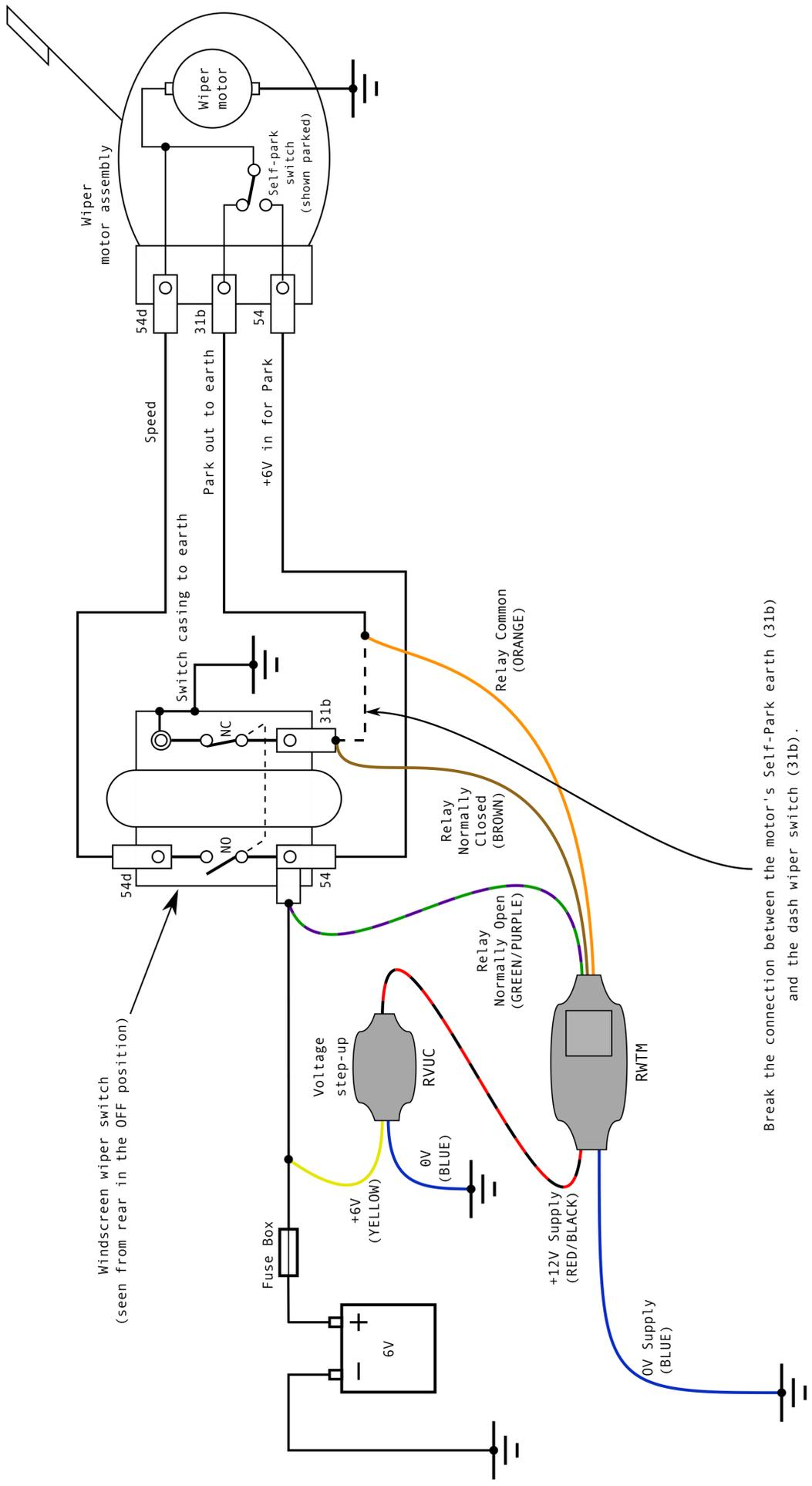
Break the connection between the motor's Self-Park earth (31b) and the dash wiper switch (31b).
